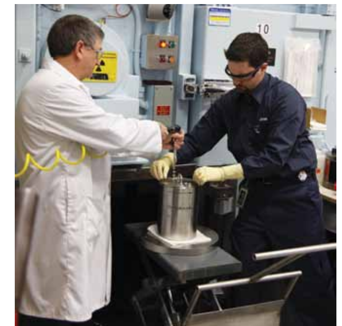
Nordion employees prepare molybdenum-99 (Mo-99) in its shielding container for shipment.
